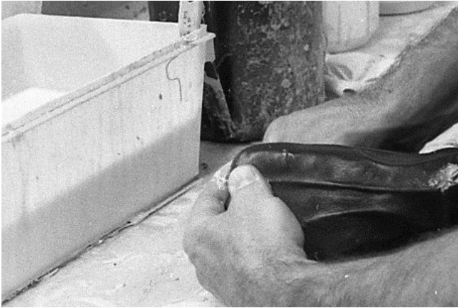
157 Ditto, and pull it tight over and around top and front of toe box.
