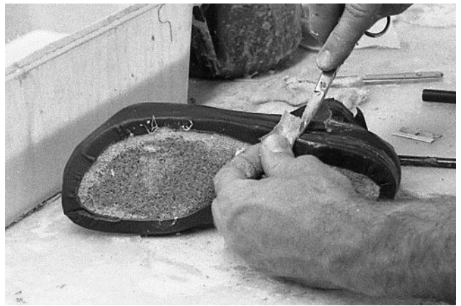
176 Trim and fold over flap of front leather to meet with a butt joint from base cords to underneath.
