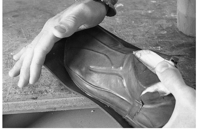
192 Use bench top to get a good press, especially in scalloped areas under medial and lateral arch.
