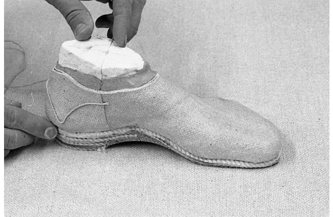
122 Design cording #18 cotton twist is applied with latex and plaster or glue. You can use any design pattern that you want. The cords will be embossed so they show through the outer leather as a raised design.
