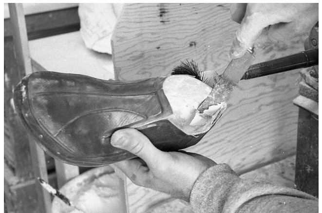
220 Scrape out with the butter knife any plaster or bits of the last from inside leather and sock.
