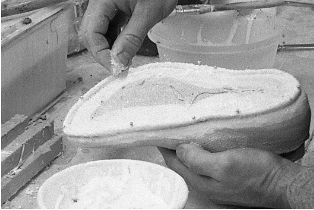
85 Apply Hydrocal® or standard plaster to speed set up of latex.
