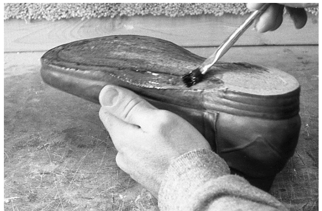
184 Apply a first coat of glue (Ubagrip®, Barge® or Reina Ortec®) to leather. Sometimes the glue needs to be thinned as it is too thick right from the can, especially as the first coat.
