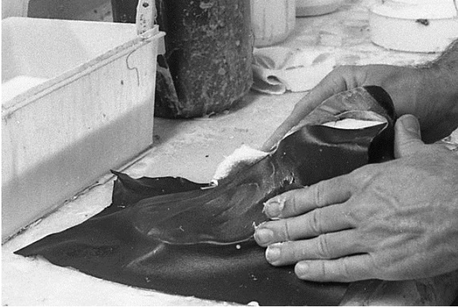
155 Ditto, and a rag is used to clean excess latex off surface of leather. Keep cleaning as you work.
