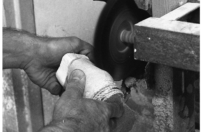
116 Monks Cloth and/or sock is best cleaned with a fine wire brush.
