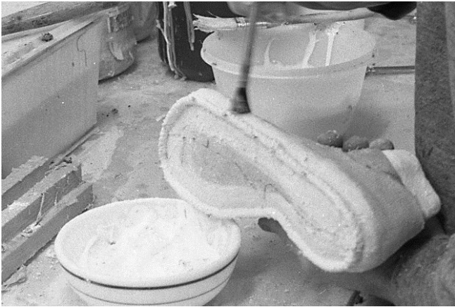
87 Extra latex is applied to make sure the bond is firm.
