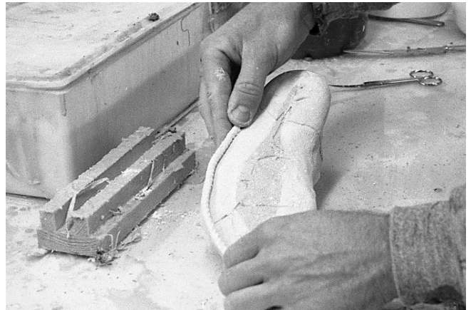
82 Apply latexed and plastered cord to bottom of last.
