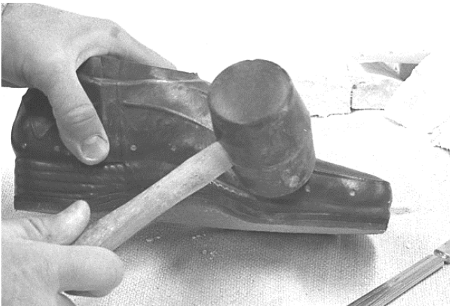
217 Because of process, last may have adhered to inside of shoe and it may need to be tapped and pried apart. Be careful if you think the cast is salvageable for reuse. The less damage to the last, the better it will be for reuse.
