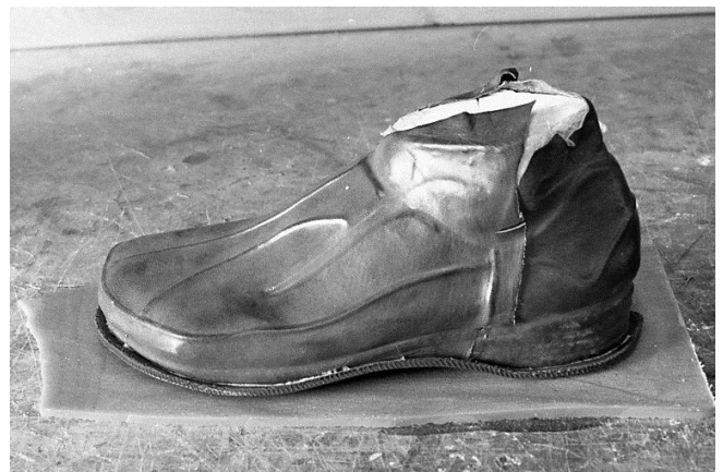
196 When glue is appropriately dry, place shoe on outer sole.
