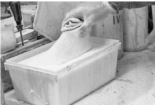
47 The whole last with sock is immersed in latex.
