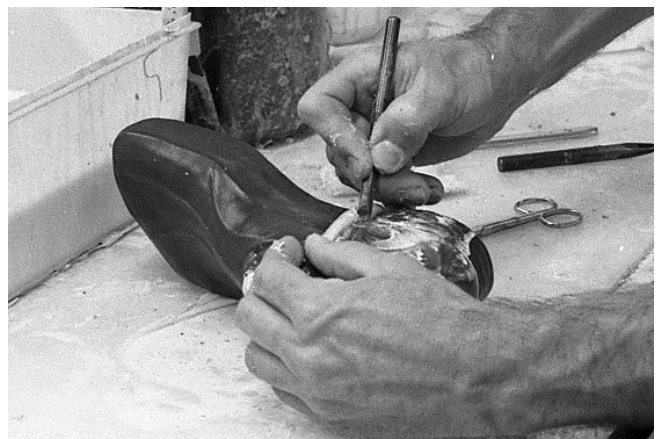
166 Use a scratching tool with 3 or 4 closely spaced needles to roughen the back leather, which will be under top or front leather when pressed and bonded.
