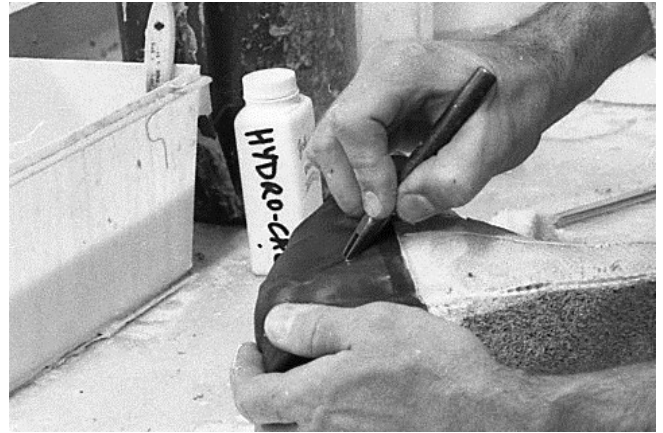
144 Leather is tooled with a forked or slotted point tool to press both side of leather against design cords.
