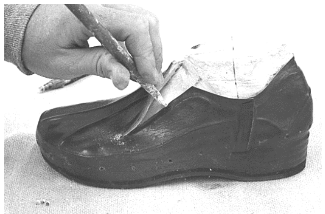
214 Use a good heavy duty, large size screwdriver and hammer to punch into and break last.
