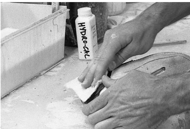
147 A rag is used to press leather into shape, and clean excess latex from surface in order to avoid staining of leather as it dries (especially light colored leathers).
