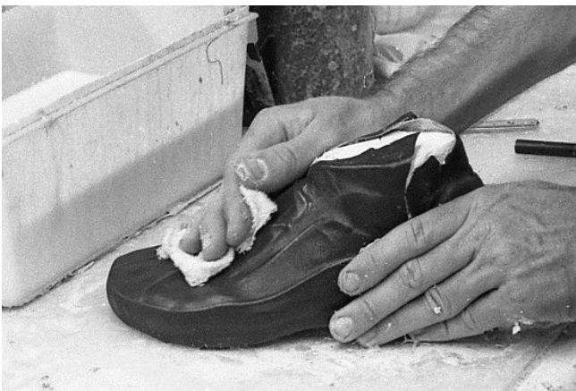
177 Press, mold and clean leather.
