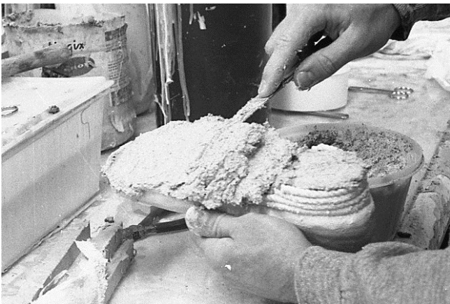
105 Apply liquid mud (soft rubber butter).
