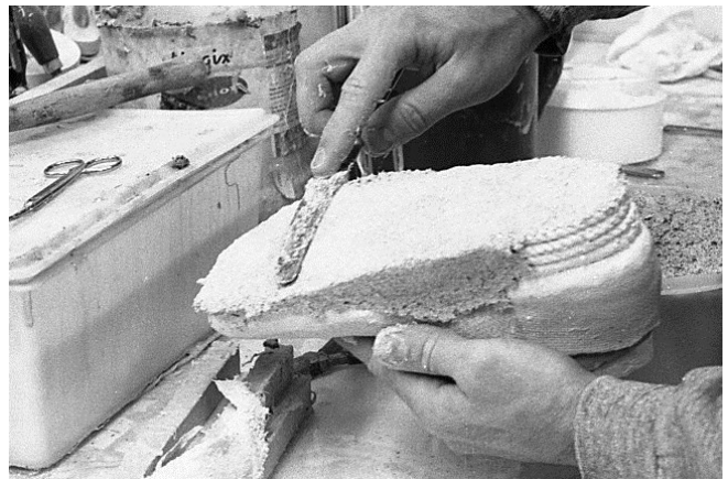
106 Rough finish base using water and/or latex on butter knife to produce a smooth desired shape.
