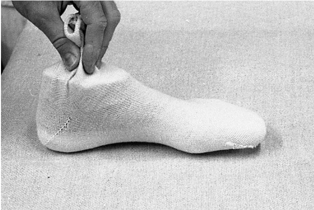
45 The sock is snugged up (not too tight—not too loose).
