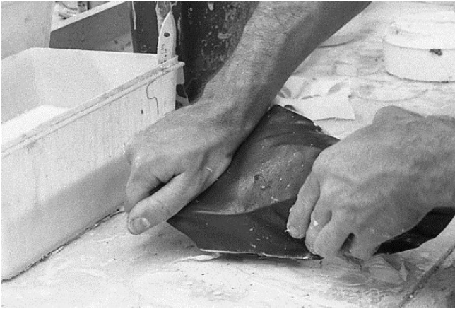
161 Stretch, press and hold front leather. Keep working the leather as you mold it to the shape of the shoe.
