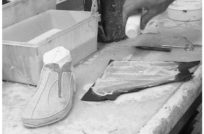
134 Hydrocal® is sprinkled onto the latexed leather.
