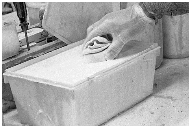
48 The latex used is 3E6S by General Latex and Chemical (now) Poly One. The latex has been thinned to desired working consistency with distilled water.
