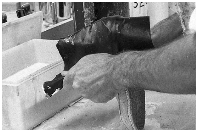
136 Heel leather is pulled and stretched around back of shoe.
