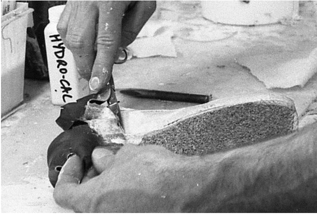
137 Front edges of heel leather are trimmed.
