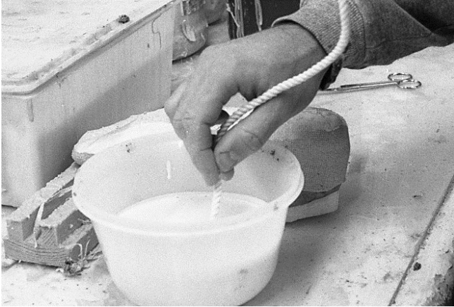
79 Soak or dip 1/4" or 3/16" cotton cord (rope) in latex.
