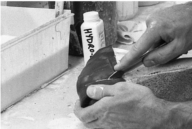
145 Leather is tooled to make it conform with good bonding and design.
