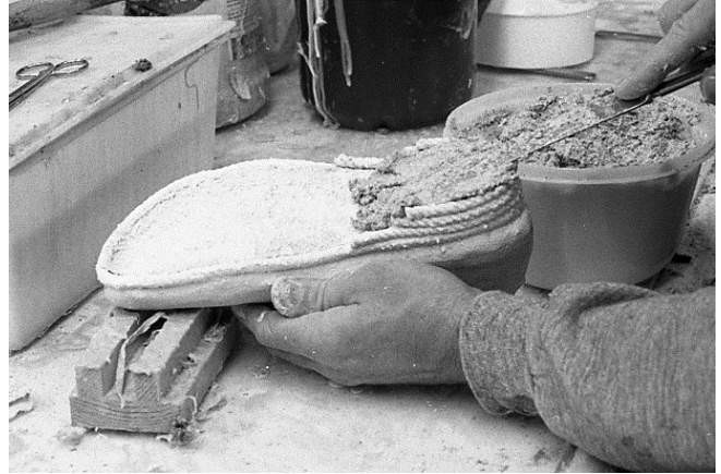
104 A mixture of mud is made and applied to build a semi-flexible base between the contours of the foot shape and the walking surface.
