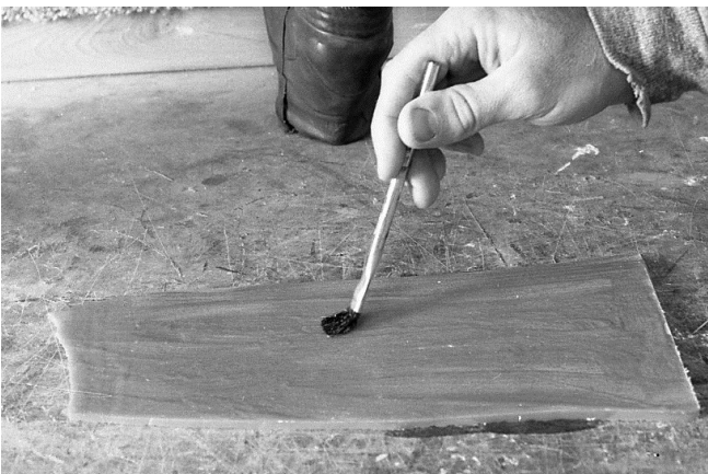
195 Apply glue to outer sole and let glue dry to tack free or longer for a better bond. The strongest bonds will be when all of the solvents have evaporated away.
