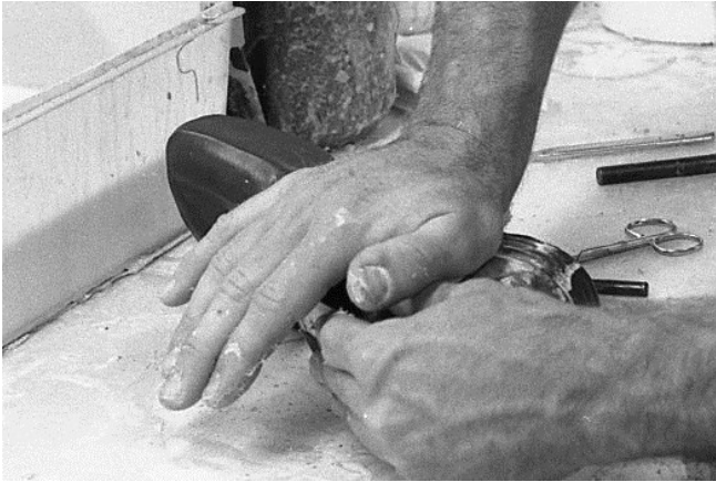
167 Press and hold front flap so it starts to bond to back leather.
