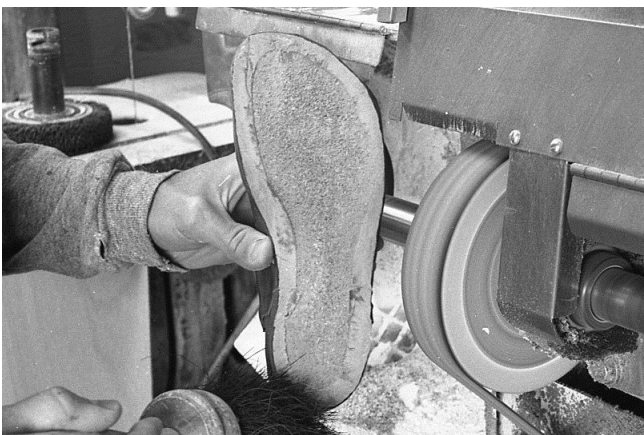
183 View of a good sanding of bottom of leather.
