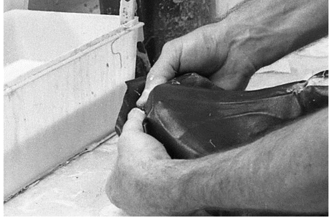
156 Leather is stretched, pulled and smoothed along sides and down under to bottom of shoe.
