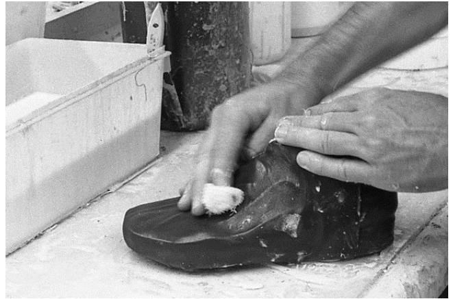
162 Clean excess latex from outer surface of leather and press out any air bubbles under leather.
