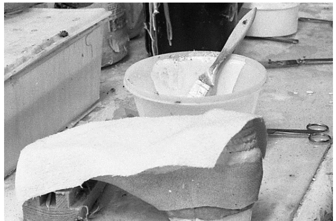
96 Once all layers of cords have dried, a piece of oversize terry cloth is cut.
