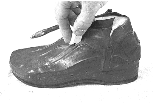
213 Cut lace opening with single edge razor blade.
