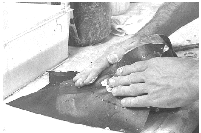
154 Leather is stretched, pressed, smoothed and molded to top of shoe.
