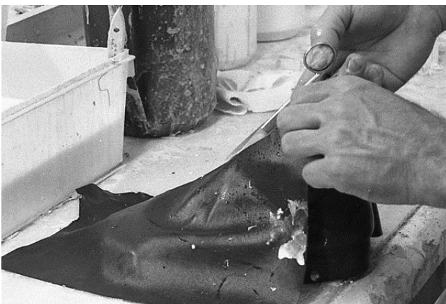
153 Leather is placed over shoe and center of leather is cut down to just above shoe top.
