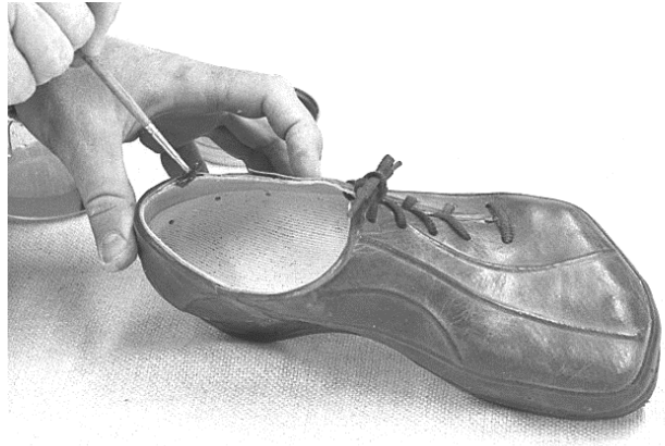
236 Glue any shoe edges where inner and outer leather have not bonded together adequately.
