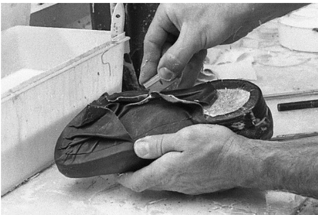
171 Cut excess front leather off bottom with a single edge razor blade. Leave about 1/4 to 1/2" inside the outer edge of shoe base.
