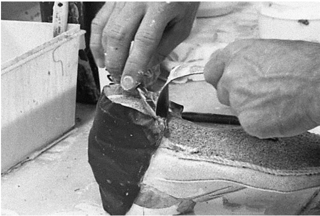
139 Bottom of heel leather is trimmed about 1/2" above base of shoe.
