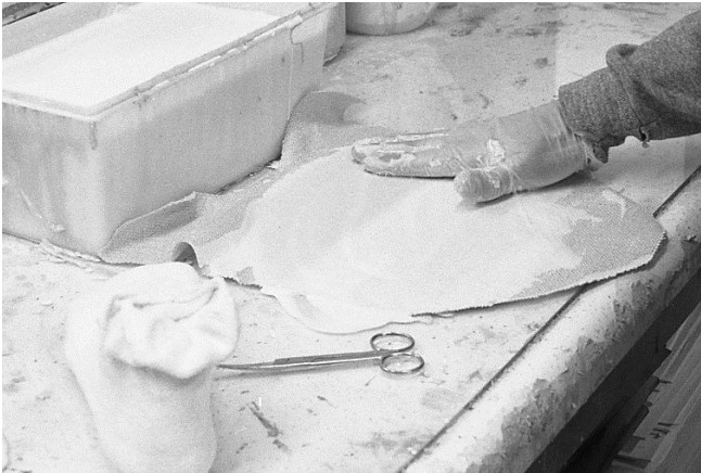
57 Latex is evenly distributed onto Monks Cloth. The nicest scissors for this kind of work are Miltex mayo operating 5.5" sharp CVD 5-116.
