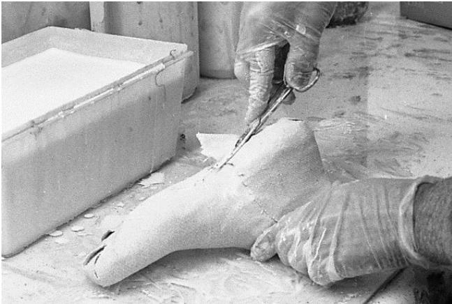
69 Fold and trim Monks Cloth to form a nice smooth heel counter (stiffener).
