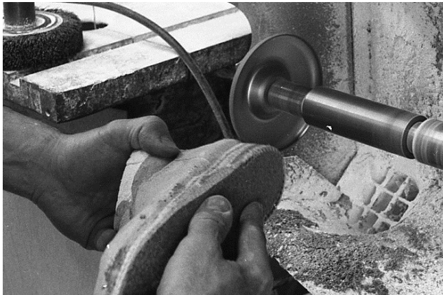
115 The top of shoe is cleaned above cord base.
