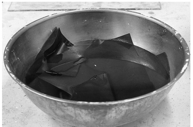
130 The outer leather can be soaked in water or latex. It can be soaked as required to get it soft and stretchy (usually 10 to 20 minutes).
