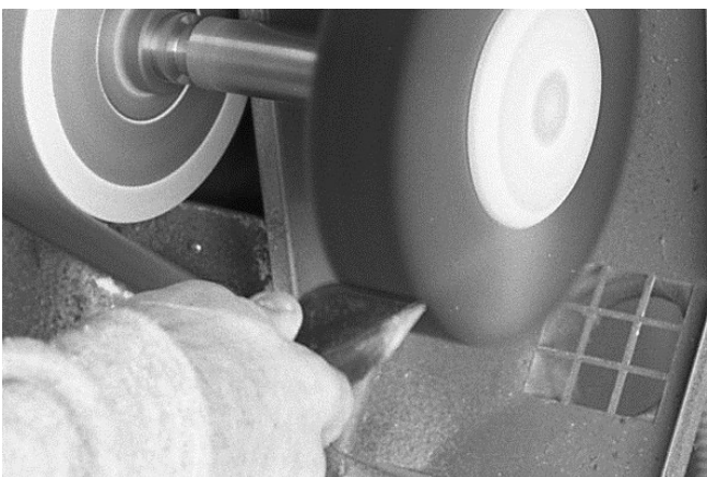
207 Polish shoe by using a hand application of Lincon® or Kiwi® paste wax polish and/or as pictured, a Renia® polish stick applied to polishing wheel.
