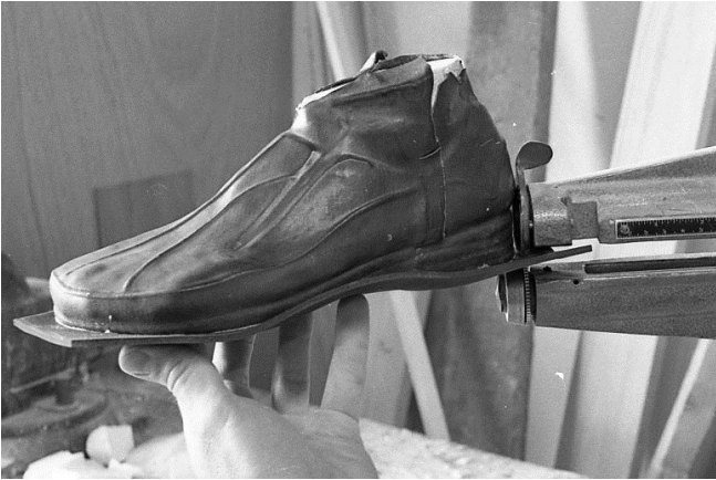
193 Trim off excess midsole with cutting machine or hand held knife.
