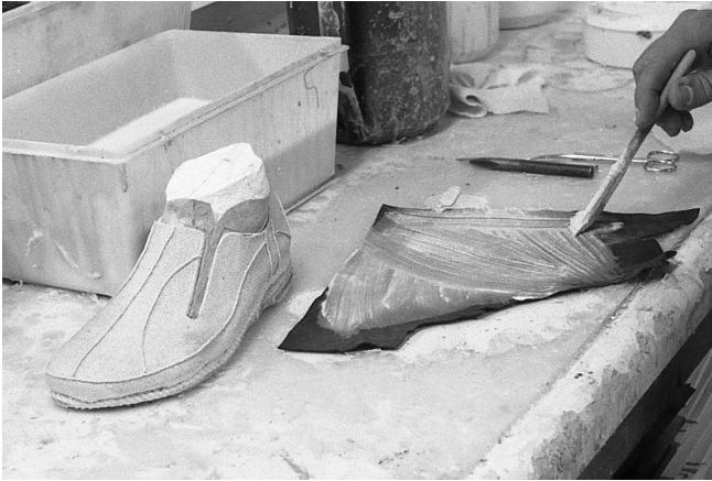
131 Excess water or latex is removed. Then, leather is placed on a glass surface and a coat of latex is applied with paint brush to underside of leather, which will become molded and bonded to shoe.
