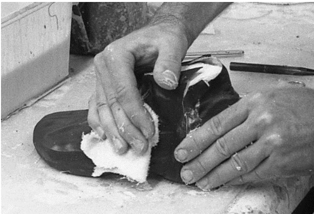
175 Clean, press and mold leather.
