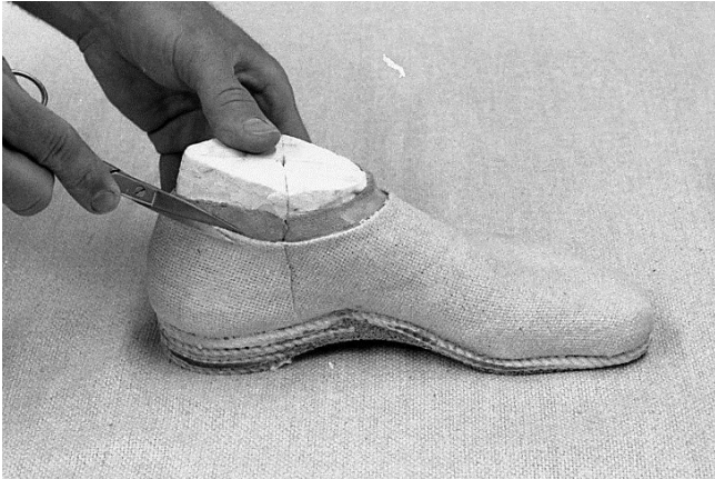
121 Shoe top Monks Cloth and sock is trimmed to cord which was used to design top of shoe.
