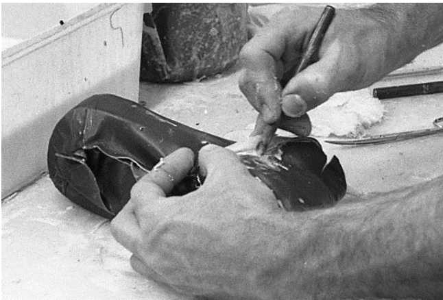
169 Use a scratching tool to roughen back leather which will be under front leather when bonded.
