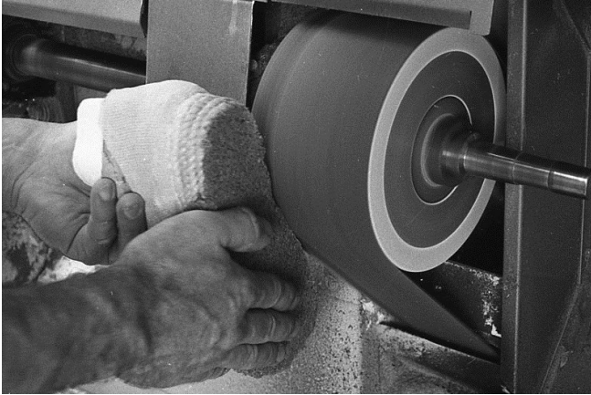
107 After one to three days of drying sand the excess of hardened mud mix on a belt sander to shape as desired.
