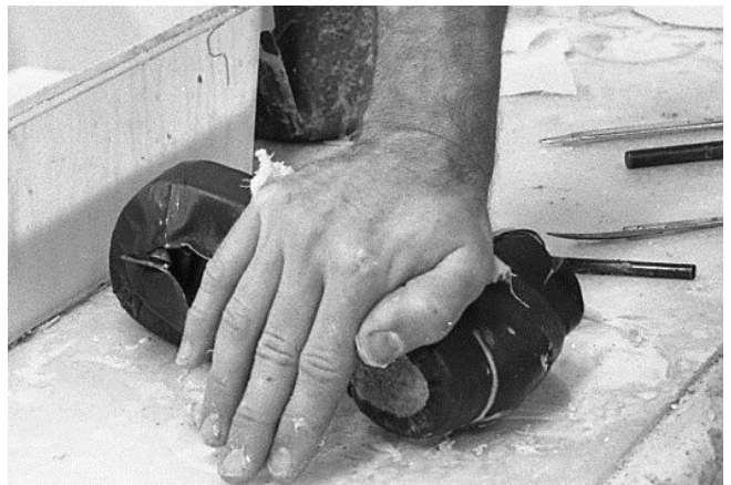
170 Press and hold front flap so it starts to bond to back leather.
