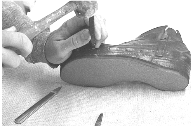
210 Punch in base perforations with a #3 punch.
