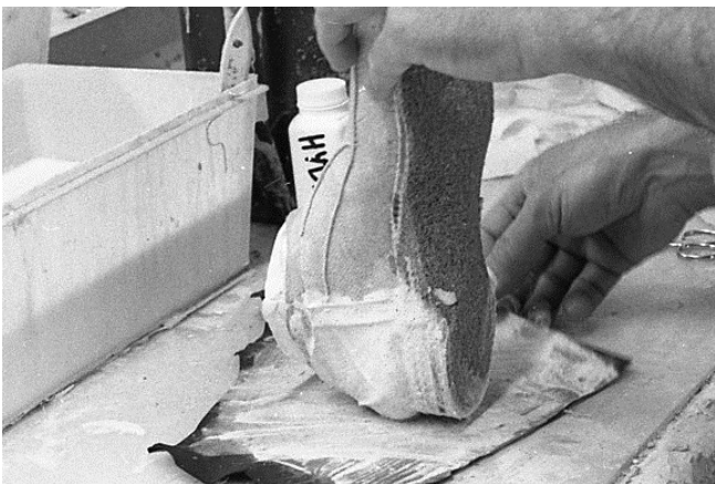
135 Back of shoe is placed on heel leather.
