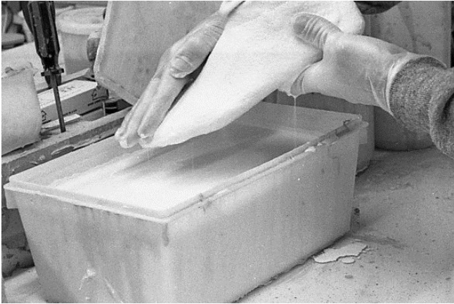
49 Excess latex is removed.
