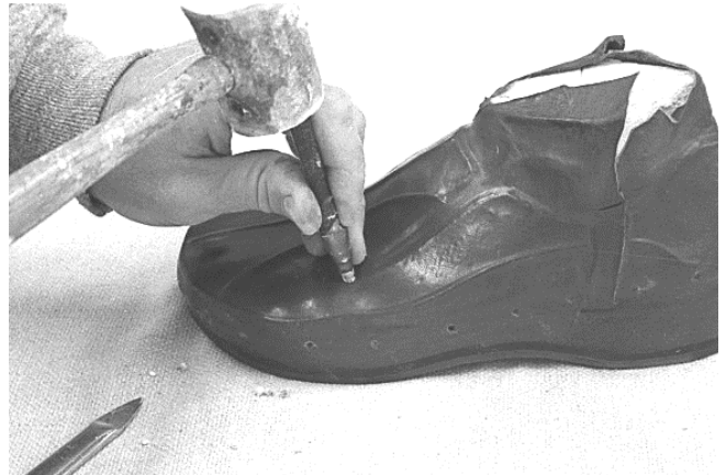
212 Punch bottom of lace opening.
