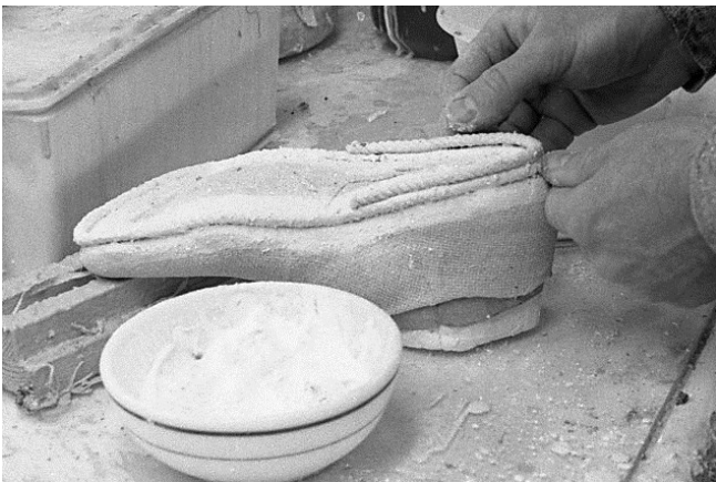
89 Three heel cords are applied, latexed and plastered.
