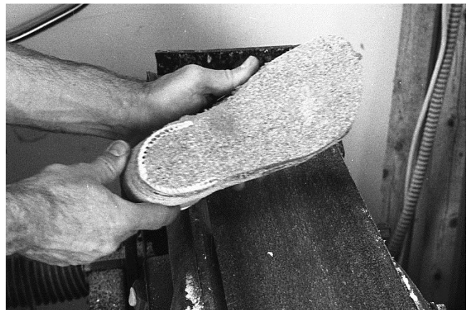
110 Proper grinding is flatness from back of heel to ball of last (foot). Stop when you see terry cloth at ball of foot. If you are uncertain of exact measurements of thickness of base, poke a needle into base until you feel hard plaster of last (cast).
