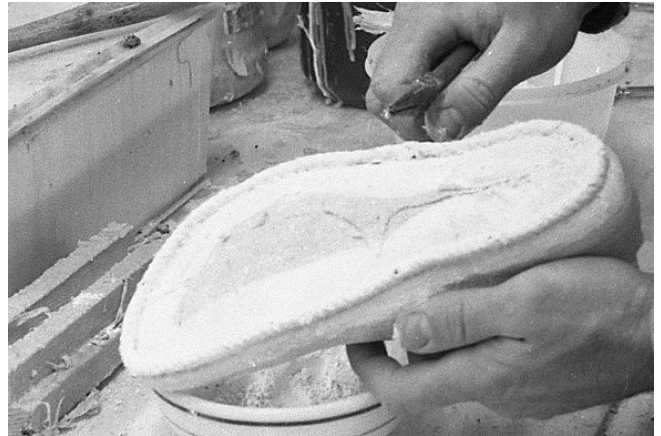
88 The cords should be flush with the outside edge of last to give a normal and functional base.
