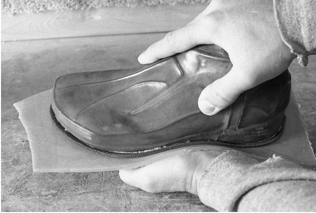
197 Press mid and outer soles together.
