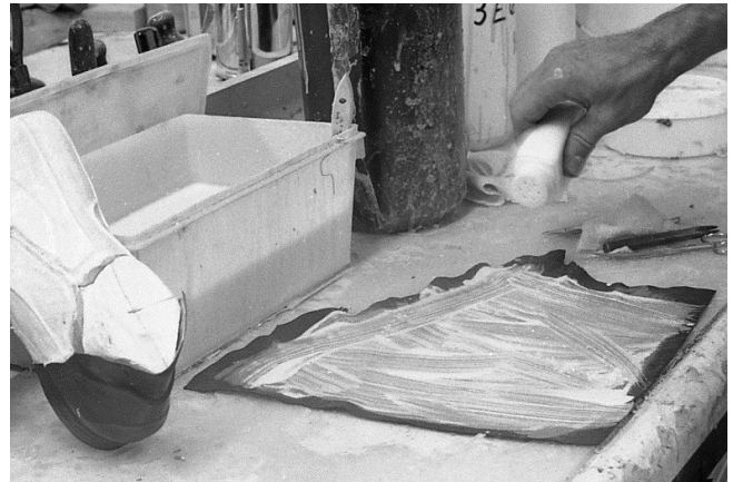
152 Hydrocal® is sprinkled over latex.
