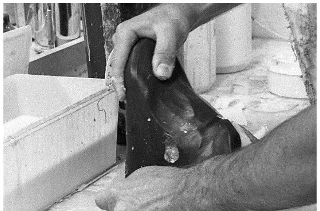
160 Keep pulling, tucking and folding leather toward back to beyond front seam of back leather.
