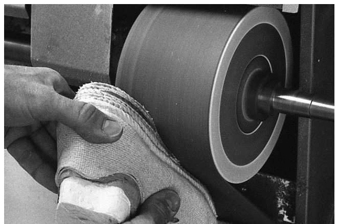
118 The lateral area under arch is usually beveled or scalloped to achieve a graceful looking shoe with some flexibility of arch.
