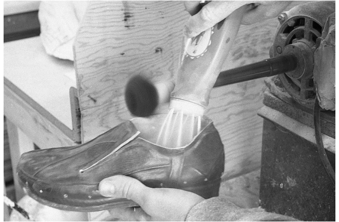
224 Add talcum powder to help the clean out and keep brush bristles from loading with latex and rubber cement.
