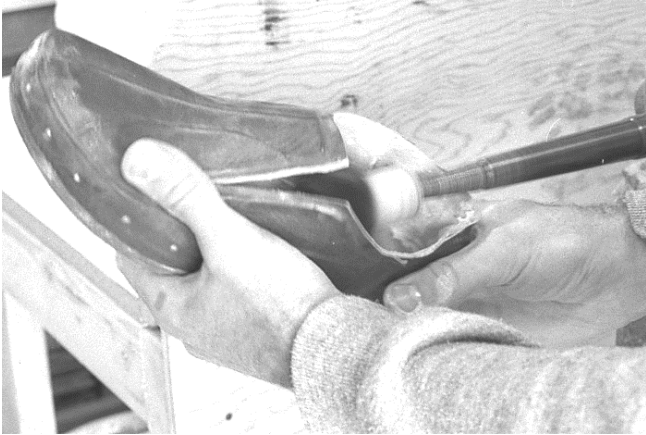
221 Use a Cocker-Weber® toe brush to clean out inside of shoe. Cocker-Weber.com 1-800-497-4541. 13RC 2.5" cup brush 3 row "toe brush". And, B27 and B29 dental lab wheel brushes.
