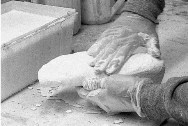
55 Mold in arch to fit sock to last.
