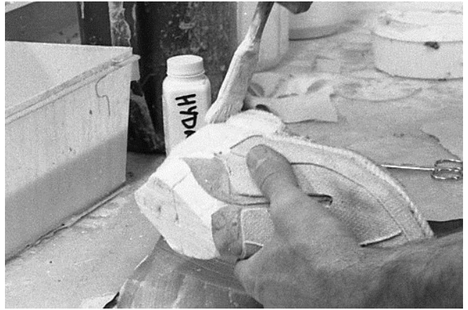
132 Latex is brushed onto inner fabric of shoe.
