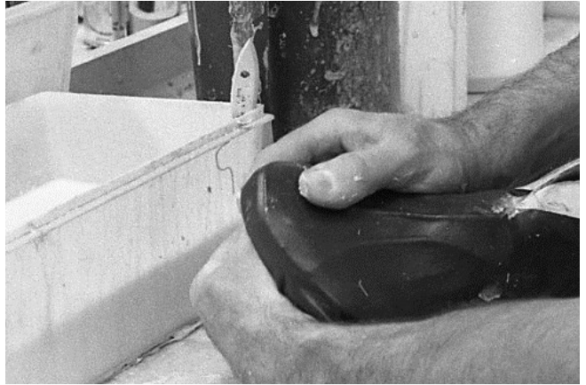
158 Tuck and fold leather under toe box and along sides.
