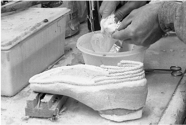
98 Excess latex is pressed out of terry cloth.
