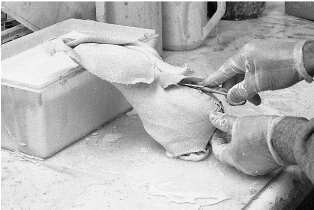
63 Fold and trim latexed Monks Cloth to fit bottom of last.
