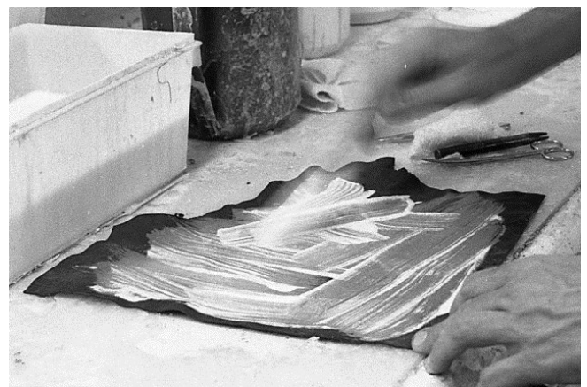
148 Front leather is placed on glass with outer surface down and inside surface up. Latex is brushed onto leather.
