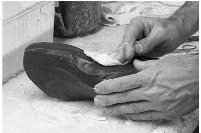
164 Clean and help the bonding areas under the arch with pressure and time until the leather conforms to the contours of the shoe.
