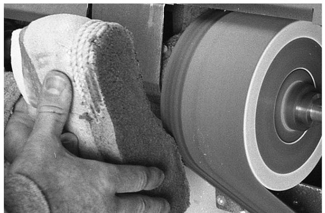
106 After "mud" has dried one to two days, it is lightly shaped and sanded smooth on the rough 24 or 36 grit sanding belt. If the "mud" deforms while sanding, the "mud" needs more time to dry.
