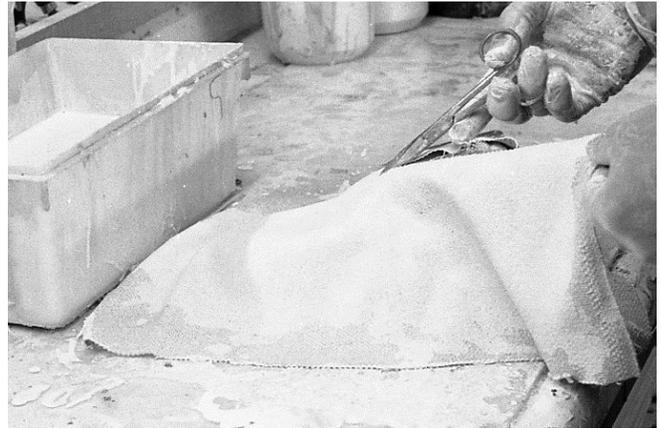
134 Front Monks Cloth is placed over shoe and center cut is made to top of shoe.
