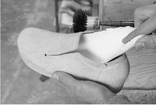
167 Insert is placed back into shoe.
