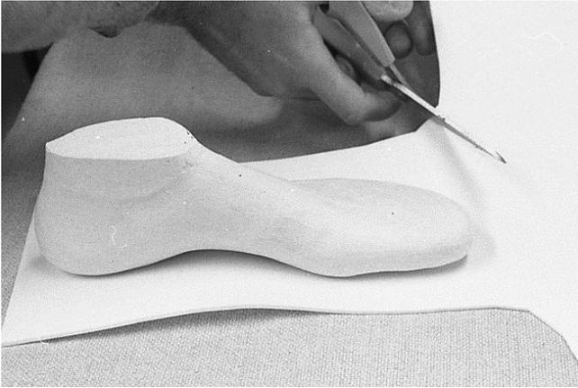
1 1/8" Pe-Lite® (3mm) is cut from sheet to make insert for foot bed inside of shoe.
