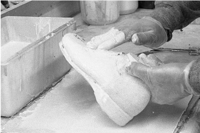
133 Latex is applied to front Monks Cloth by dipping and then hand spreading. Then latex is applied to front of shoe.
