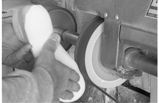
6 Pe-Lite® is sanded so edges meet the perpendicular edge of last.
