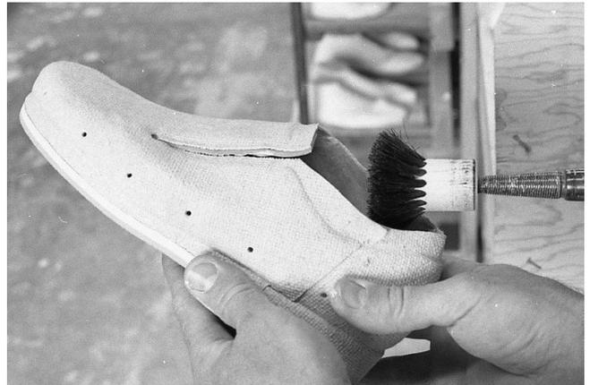
164 Inside of shoe is cleaned with a toe brush.
