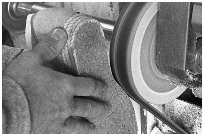
112 The outside of cord/mud base is sanded to the finish as desired.
