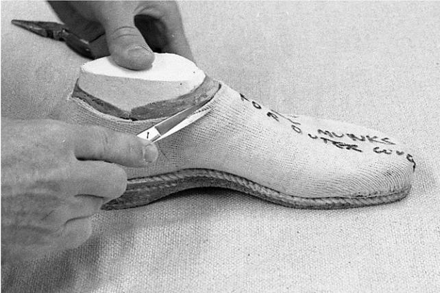
121 The waste material is removed to design cord.
