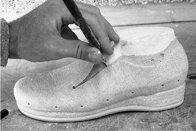
161 A large and long shanked screwdriver is used to crack the last and pry out pieces.
