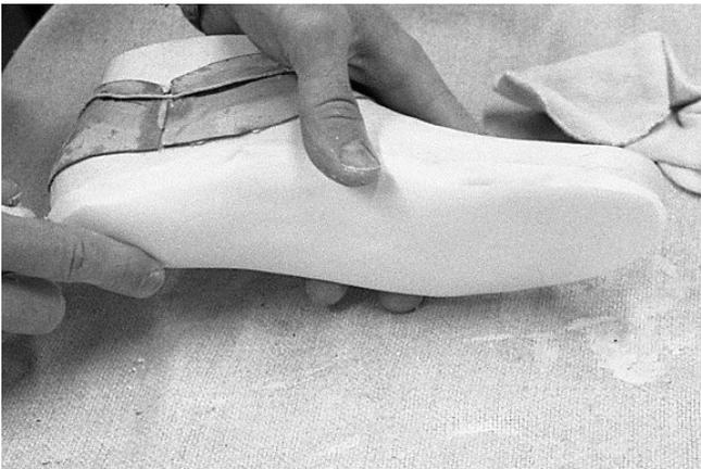
31 Insert is put on proper position on last.
