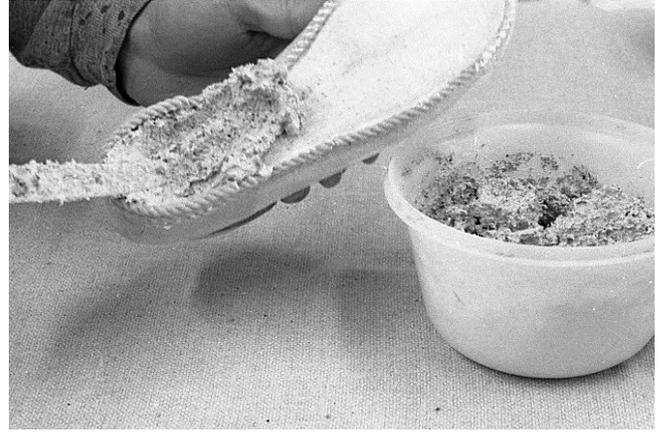
96 Notice the free standing consistency (lack of too much slump) of mix. The "mud" is placed and pressed into position inside cords.
