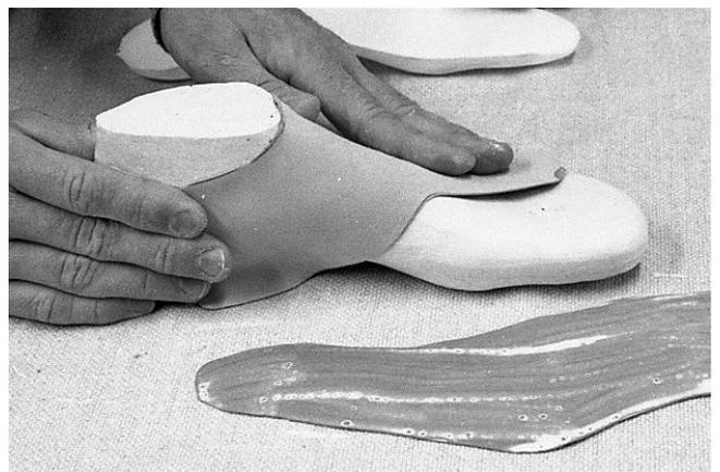
16 Latexed surface of lining leather is placed on last and pressed into place when wet.
