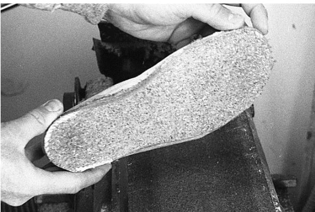
111 The bottom has been sanded flat from heel to ball and ball to toe.
