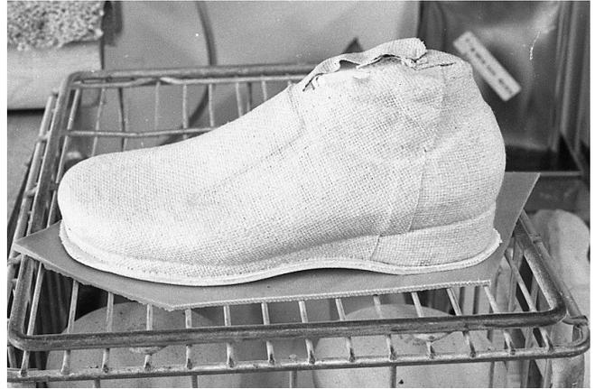
152 After adhesives dry, soling materials can be fit together.
