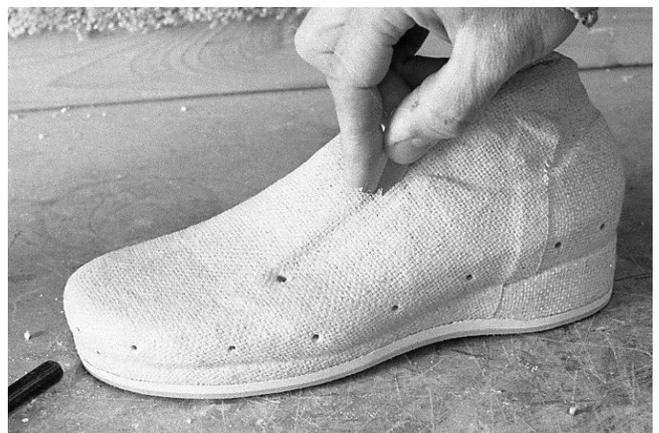
160 A single edge razor blade is used to cut lace opening.
