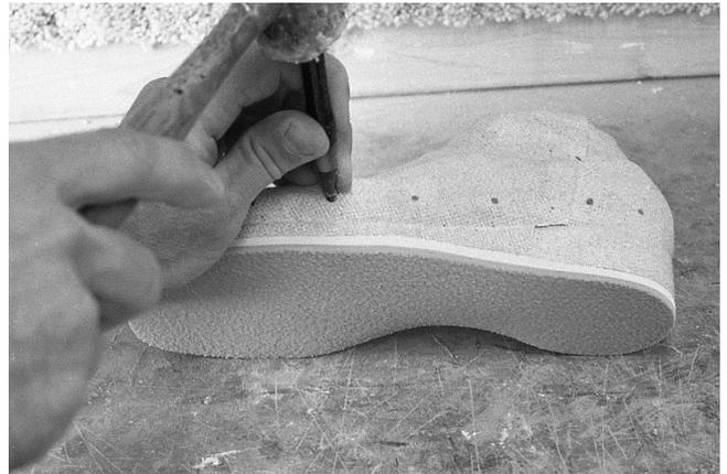
158 Base perforations are punched with a #3 punch.
