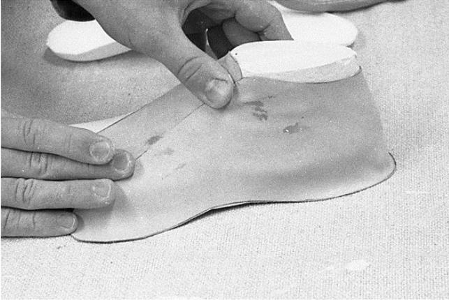
17 Second lining leather piece is placed on last and pressed into place.
