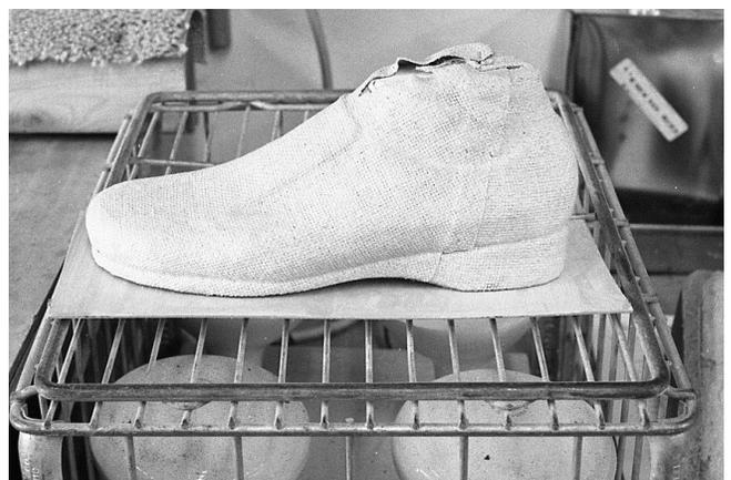
148 After drying, some adhesives can be reactivated by heat or heat can be used to drive off any leftover solvents so as to produce a firmer bond.
