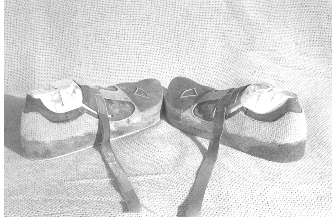
14 Another sandal in the making, which required a very soft covering over the toes (no sock only very thin lining leather and a thin soft outer leather).
