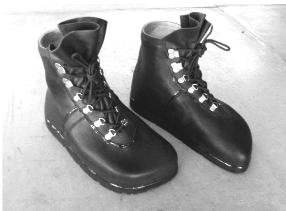
125 A pair of hiking boots with two hooks on top. The shiny spots around bottom of leather and sole, tongue and side seams, is a bead of Freesole® sealing that is reflecting the light.
