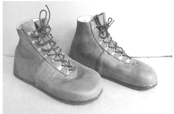
84 The finished boots. These boots are flat. No heel wedge has been used in the fabrication.
