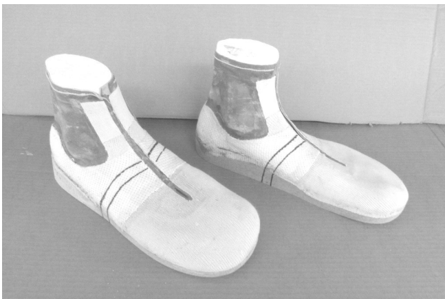
83 Additionally, this person needs softness over the front of the foot. A soft leather will help avoid deep and hard creasing on the front of the boots, especially over top of the toes.
