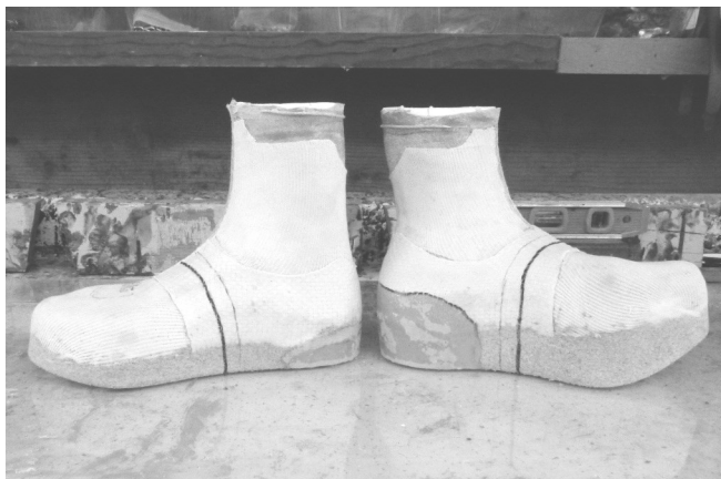
32 Fiberglass resin has been added to the heels and to the lateral side on the left boot for strength and support.
