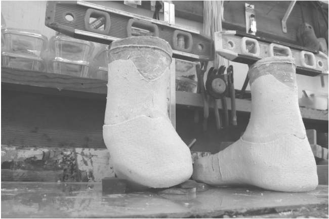
9 Two Plastazote® inserts were added to the last. Then the lining leather was applied, design cords added, socks added, Monks Cloth added and the materials were latexed.
