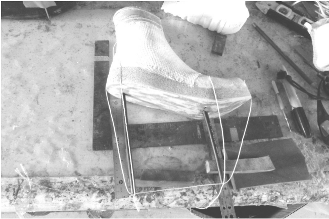
55 I used small hollow tubing to go from the fiberglass to the desired height of lift. The strings are to keep the tubing in place.
