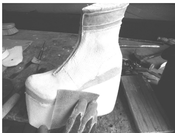
70 The foam is sanded by machine and by hand.
