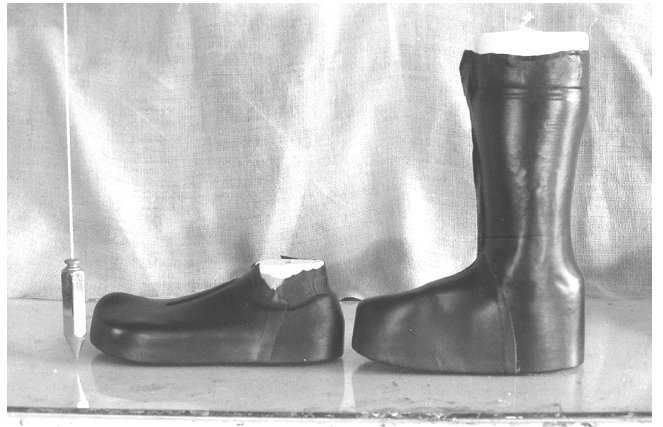
80 The front leathers have been applied.
