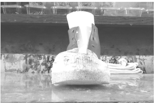
90 Not shown was the re-plastering of the front of the last to make it bigger (I was guessing again). Then the last was inserted into the stretched boot before re-"mudding" the front of the boot.
