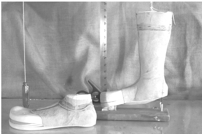
43 The top design cord of shoe has been applied.
