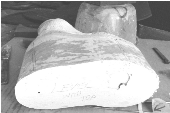
90 A fiberglass resin bottom was added and sanded level with the top of last.
