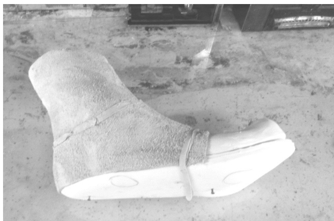
21 The back leather lining has been added. Notice I use circles around tender spots and sensitive areas to keep track of their position.
