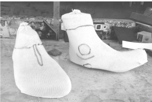
26 The leather lined last has been socked and sensitive areas marked again.
