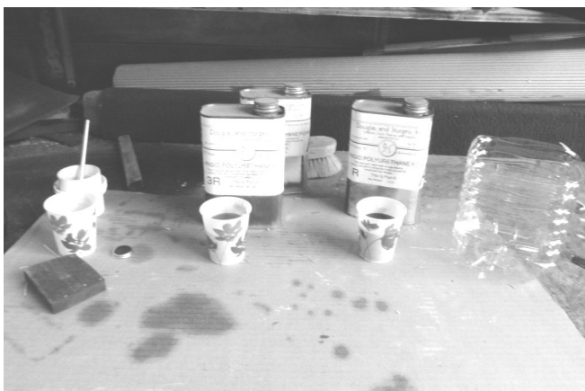
65 A two part rigid polyurethane (3# density) foam is ready for mixing. Different weights and densities are available from Tap Plastics or Douglas and Sturgess.
