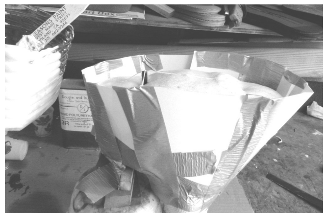
66 The foam has been mixed, poured and it has risen.
