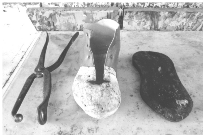
85 This time I only needed to make the front bigger again. I broke the latex bonding with thinner. Then I used a ring and ball stretcher to increase the size of the inner materials.
