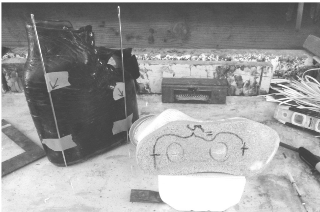
51 I have marked the position of the measuring needles
