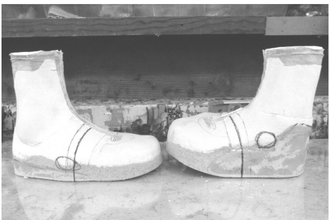
34 The position of the circle was to mark where the fiberglass resin was to be omitted.
