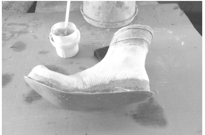
54 The fiberglass bottom gives strength and rigidity to the base. It also makes a hard and defined surface as a needle stop.
