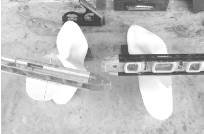
10 Ditto. Notice the use of little tapered balancing wedges on the glass surface to hold the last in a level position.
