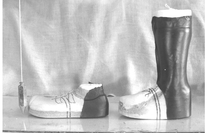
78 The back leathers have been applied.
