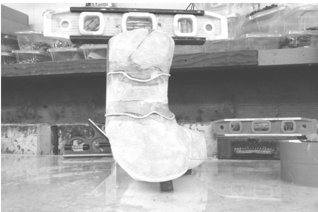
70 New inserts were made and added before the leather lining was applied.
