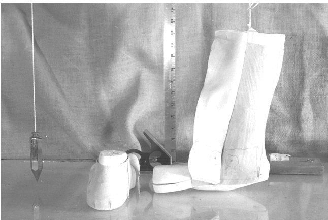
39 An additional lining leather has been applied to the boot last. The inside lining will be able to be folded back so inner padding can be repositioned at any time.
