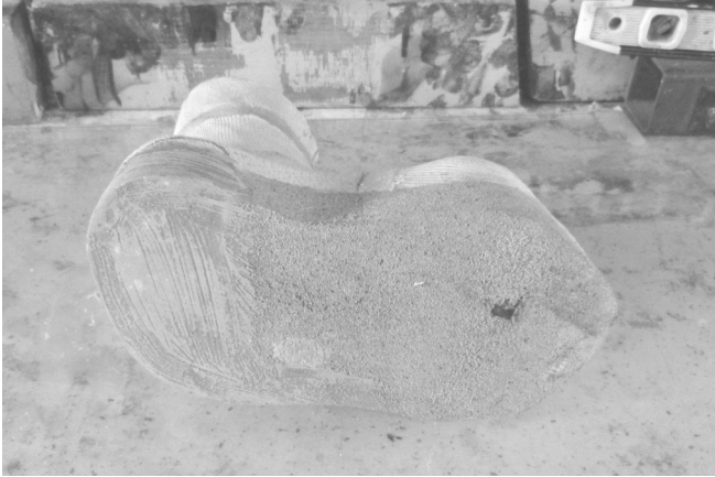
74 After sanding, the fiberglass resin was applied.
