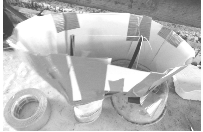
62 A shell was configured out of file folders and taped together for the purpose of holding rigid foam.
