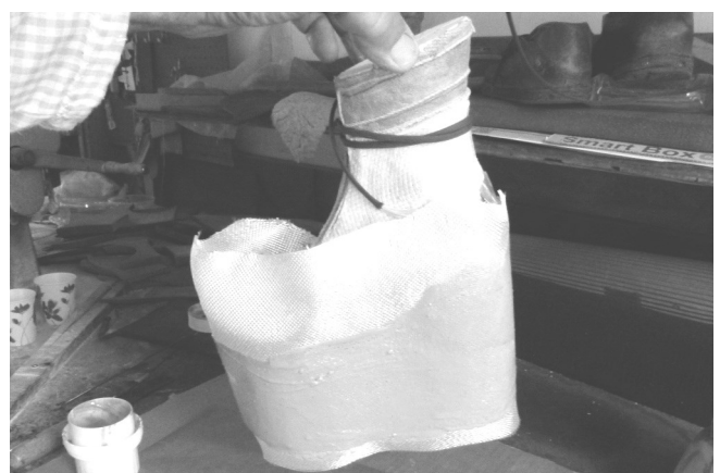
78 I apply fiberglass cloth and resin to give the outer wall of the foam strength and durability.
