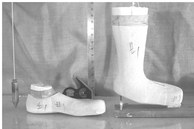
48 The socked lasts have been latexed, a heel Monks Cloth has been added and latexed.
