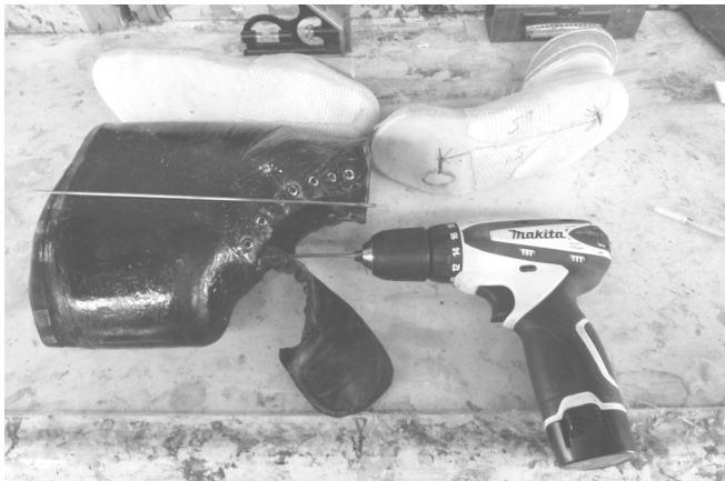
32 I drill through a “good” boot in order to insert upholstery needles and make measurements.
