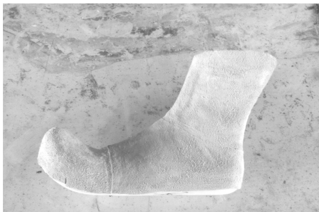
23 The front leather lining has been added.
