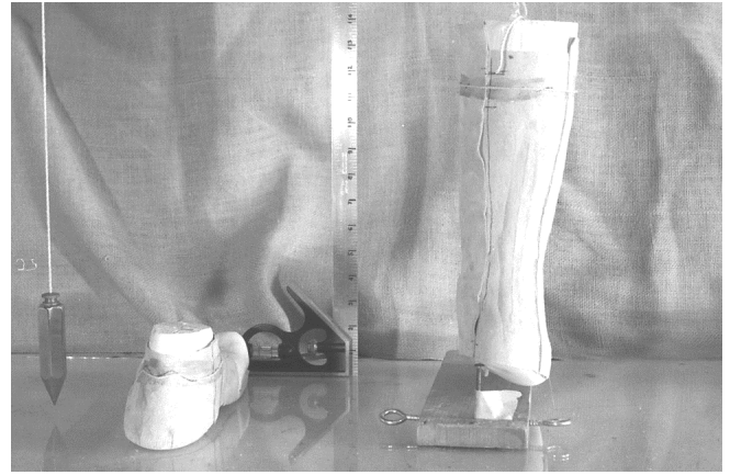
42 Back view of outer lining wrapping seam on medial side of right boot last. The alignment is re-checked and the markings for the outer edge design cords have been applied.
