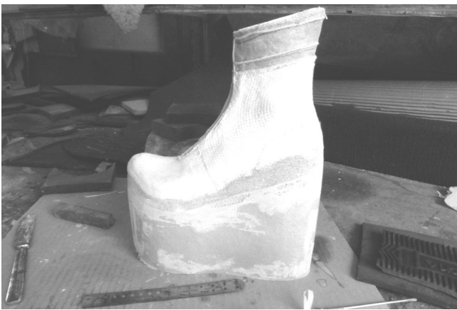
87 Final preparation of the bottom and sides of lift.
